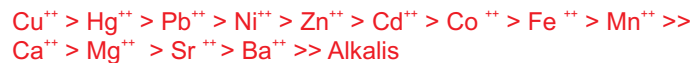
figure 4: Selectivity series of an amino-di-acetic acid (IDA)-resin. Only a selection of ions (mainly divalent ones) is given. Heavy metal ions are preferably bound.
