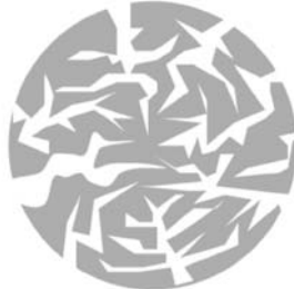
figure 1: Ion exchange resin beads contain many fine pores that fill with water. The water content of some types is up to 70%.
