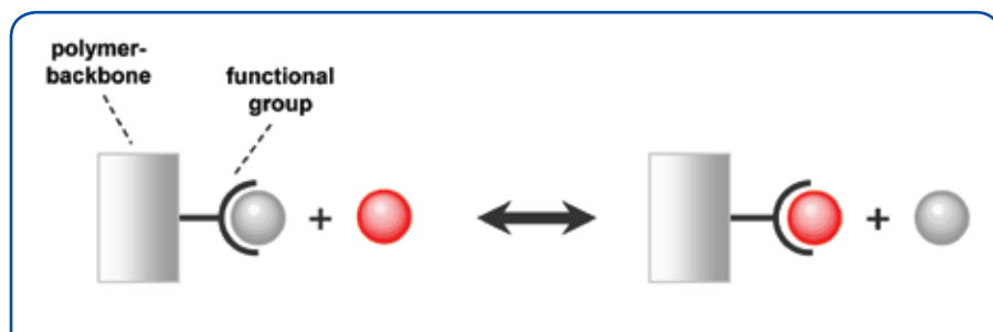
Figure 2: a fixed and a mobile ion are changing places in a so-called ion exchange reaction. This simple reaction scheme is the base for more than 500 applications involved in the purification of water and other fluid media.
