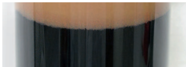
Perfect separation of cation and anion exchange resins in a mixed bed
