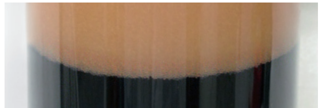
Perfect separation of cation and anion exchange resins in a mixed bed
